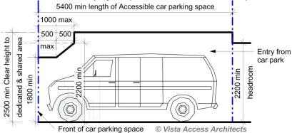
Head heights for both dedicated accessible parking space and the shared zone to be as shown above. No beams, pipes, sprinklers or any other encroachments are persmissible for the entire 5.4M width of the dedicated and shared zone as per Section shown above.
