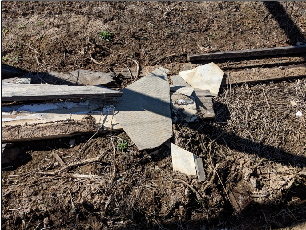
Photograph 9: Fibro cement sheeting located within the central portion of the site.
