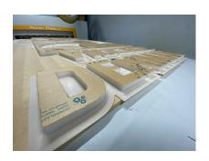
30mm Solid Opal Acrylic CNC cut with 3mm backing for attaching to panel
