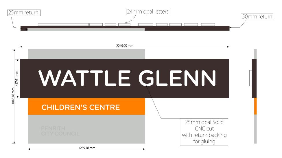
Suggested Materials: Aluminum frame with grooved and folded 3mm aluminum panels powder coated in the closest colour from the Dulux powder coating range. (Grey and the Brown)Orange to be Avery 900 series vinyl.
