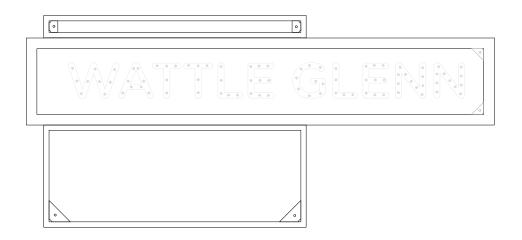
All panels to be fixed to frame work with security screws
