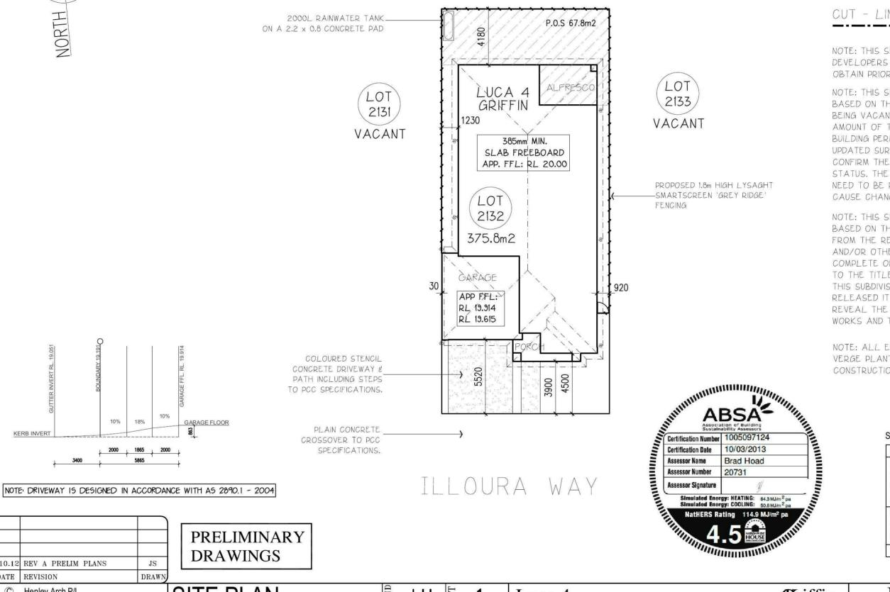
**CUT & FILL BUILDING AREA TO** RL 19.615 APPROX. TO CREATE LEVEL BUILDING PLATFORM FOR **WAFFLE POD SLAB**
