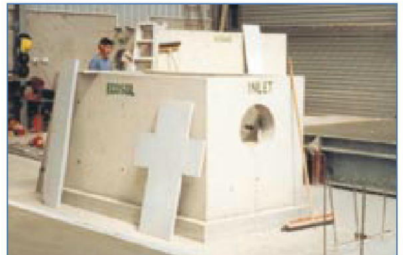
The RSF 4000 pre-cast concrete pit showing the oil and grease baffles prior to fitting
