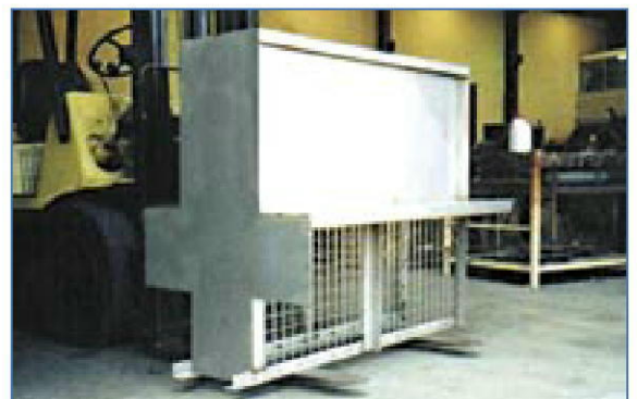
Internals ready for factory installation into pre-cast concrete pit
