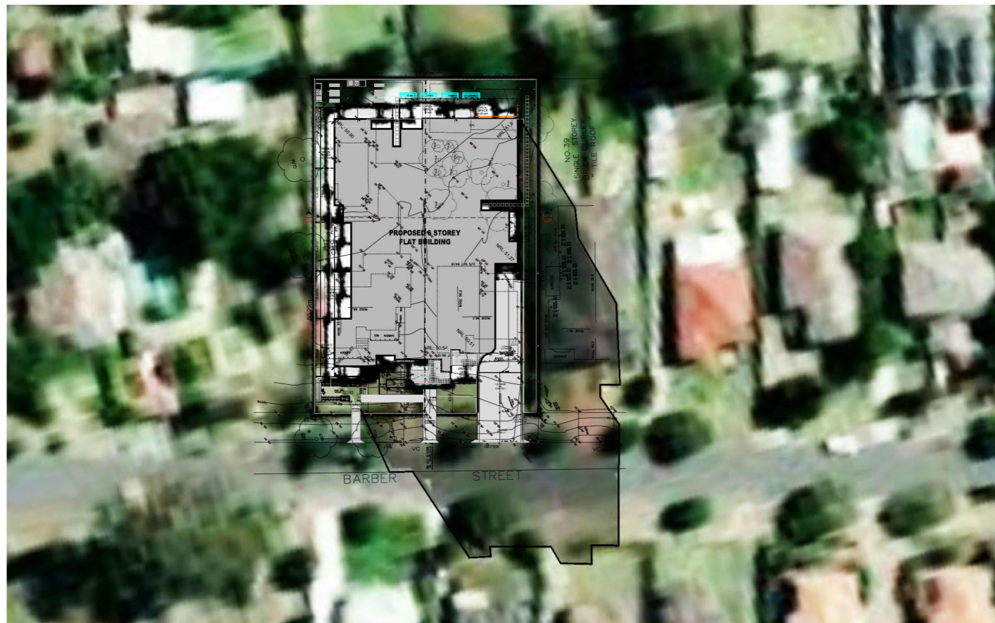
05 SHADOW DIAGRAM- WINTER SOLSTICE: 21 JUNE 01.00PM SCALE 1:800 @ A3
