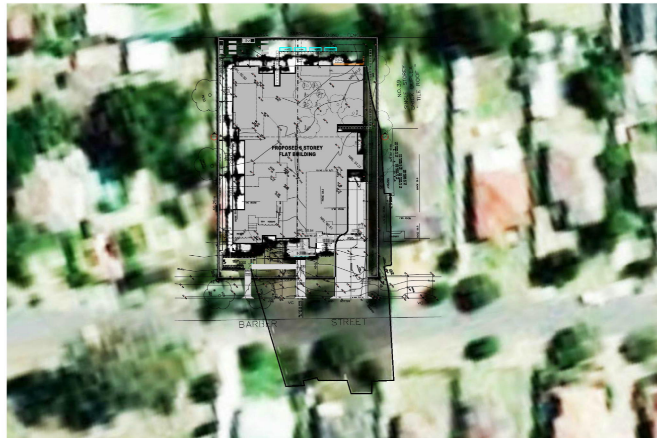
04 SHADOW DIAGRAM- WINTER SOLSTICE: 21 JUNE 12.00PM SCALE 1:800 @ A3
