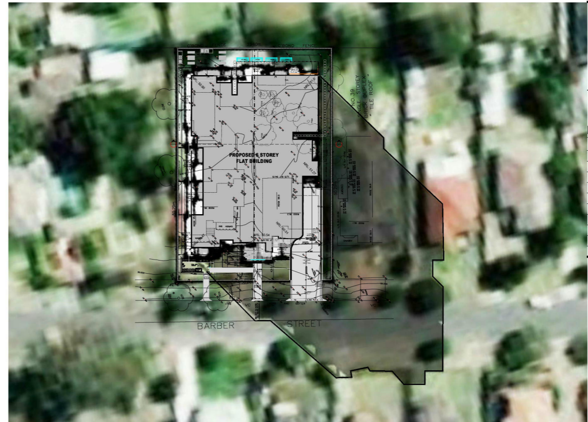
06 SHADOW DIAGRAM- WINTER SOLSTICE: 21 JUNE 02.00PM SCALE 1:800 @ A3
