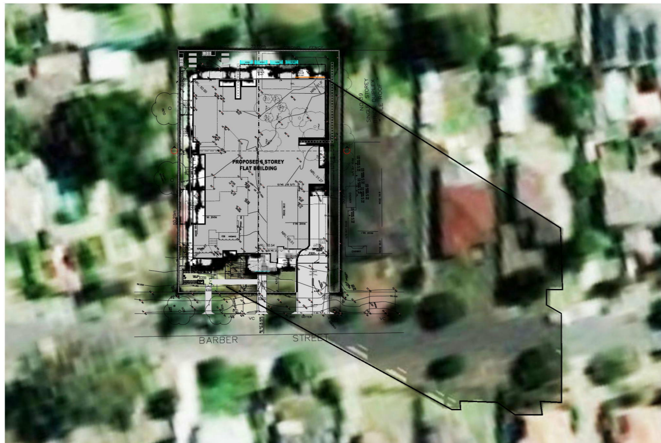
07 SHADOW DIAGRAM- WINTER SOLSTICE: 21 JUNE 03.00PM SCALE 1:800 @ A3
