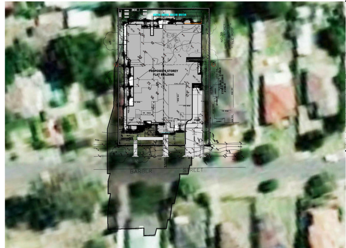
02 SHADOW DIAGRAM- WINTER SOLSTICE: 21 JUNE 10.00AM SCALE 1:800 @ A3
