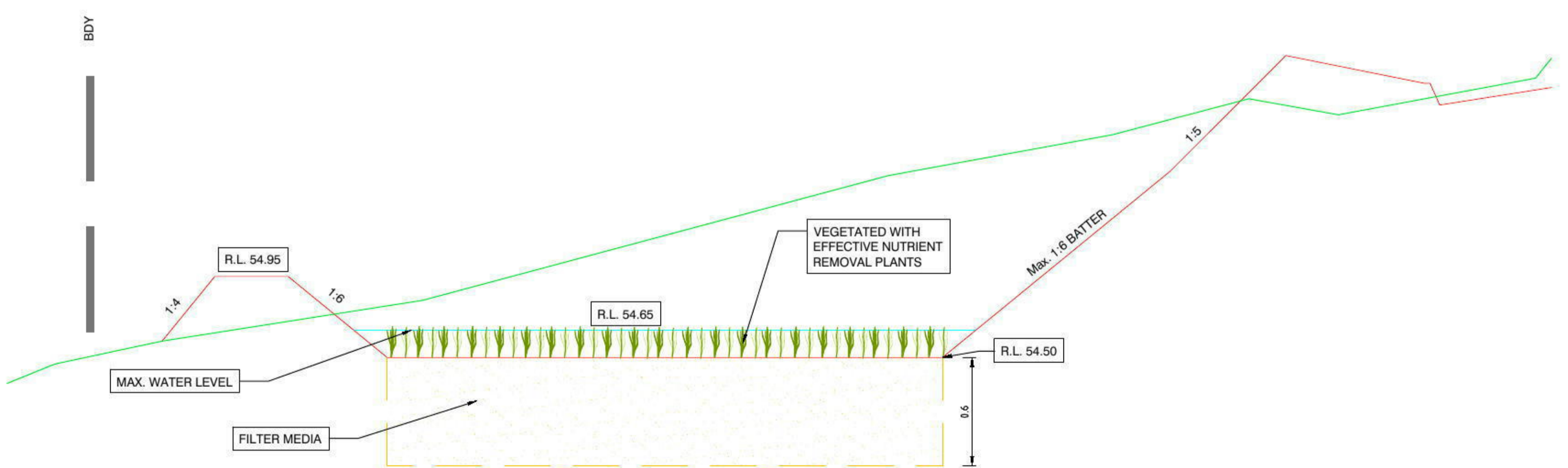
BIORETENTION TYPICAL SECTION H:1:500 V:1:100
