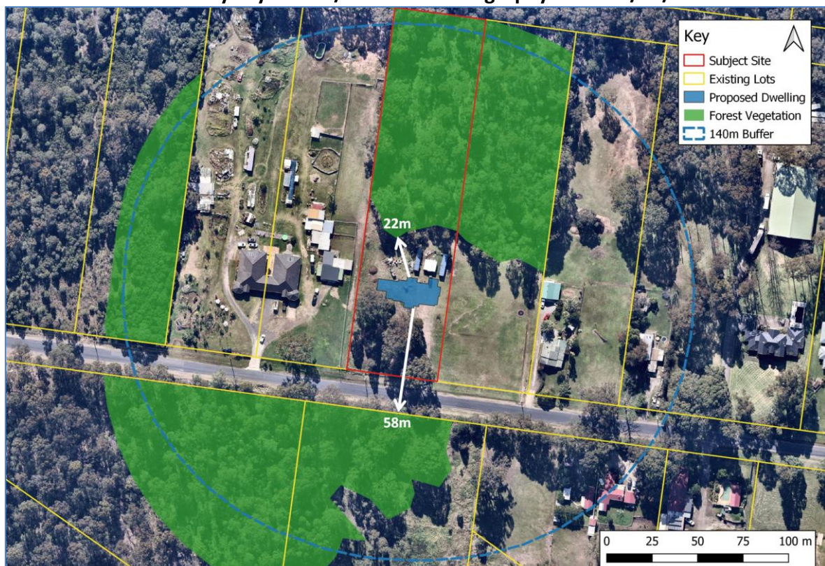
Figure 6. Hazardous vegetation affecting the subject building. Source: NearMap (2021) with overlays by BFCS P/L. Aerial Photography date: 20/05/2021
