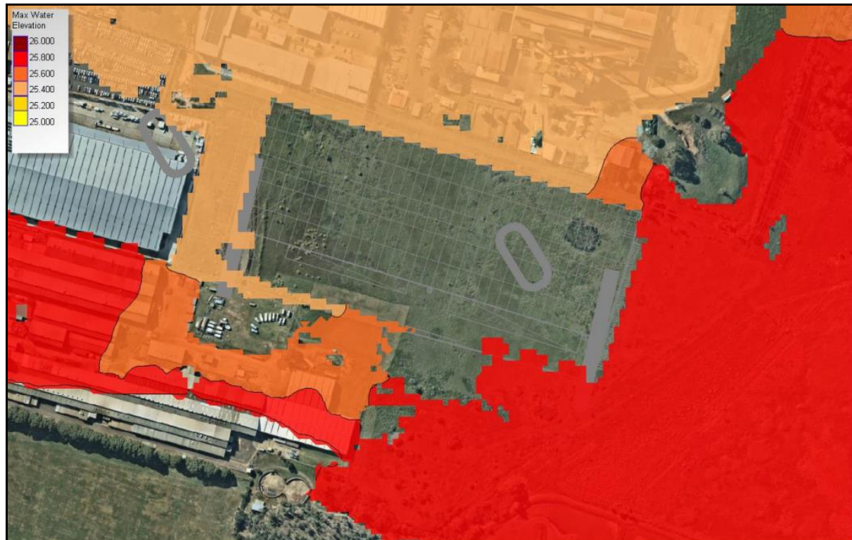
Figure F14 – 0.5% AEP Flood Level – Post Development
