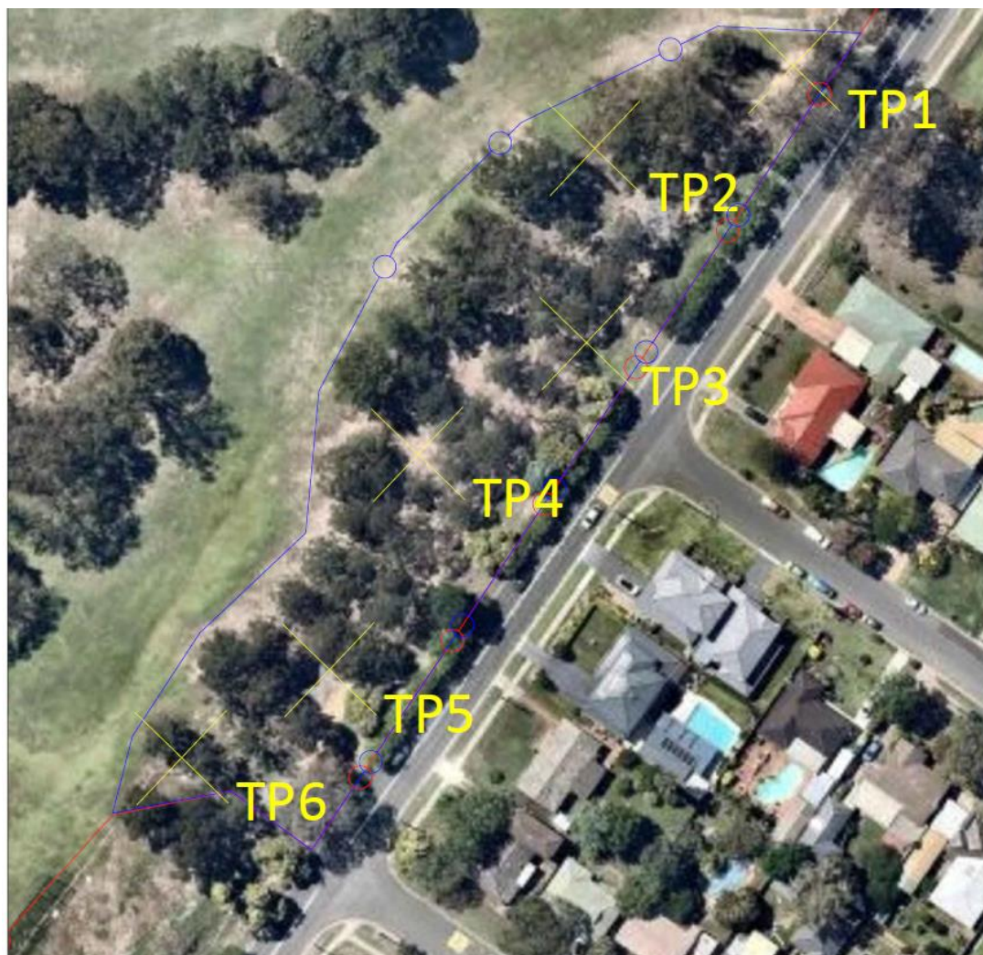
Figure 3: Site sampling plan showing location of the six (6) test pits (yellow). (enhanced image Appendix B).
