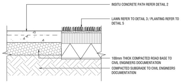
04 INSITU CONCRETE PATH / TURF INTERFACE TYPICAL DETAIL
