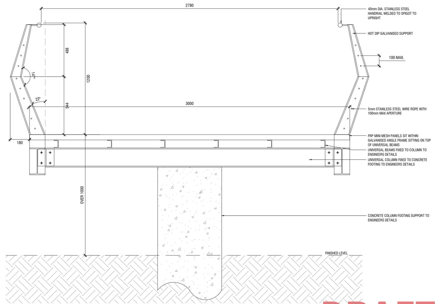
03 FRP MESH GRATING BOARDWALK / BRIDGE TYPICAL SECTION
