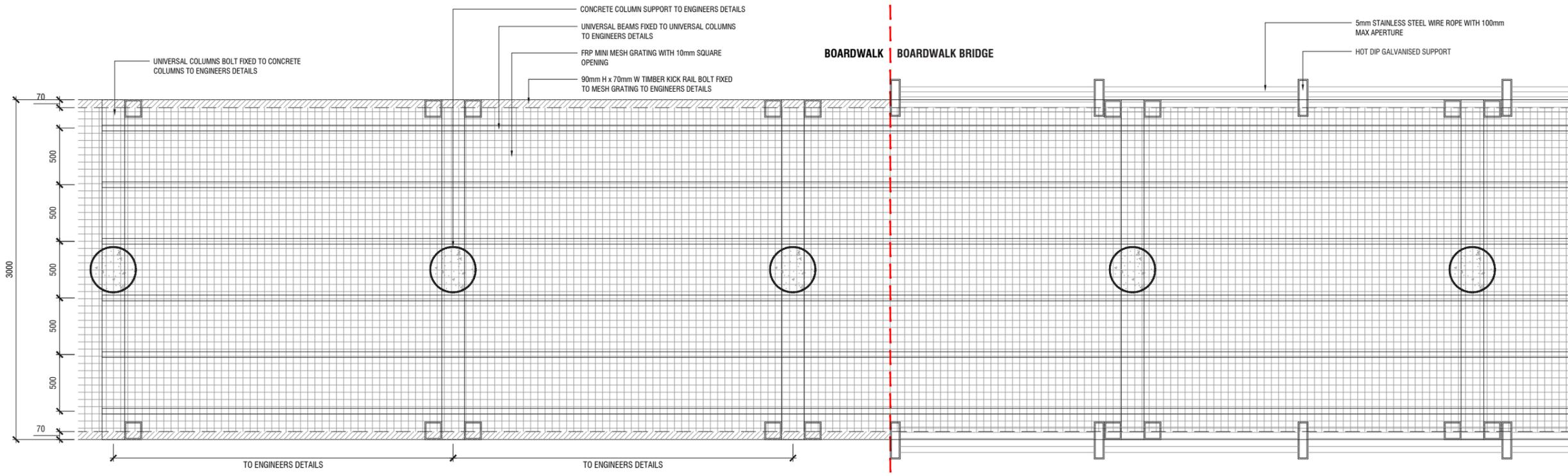
01 FRP MESH GRATING BRIDGE / BOARDWALK TYPICAL LAYOUT PLAN
