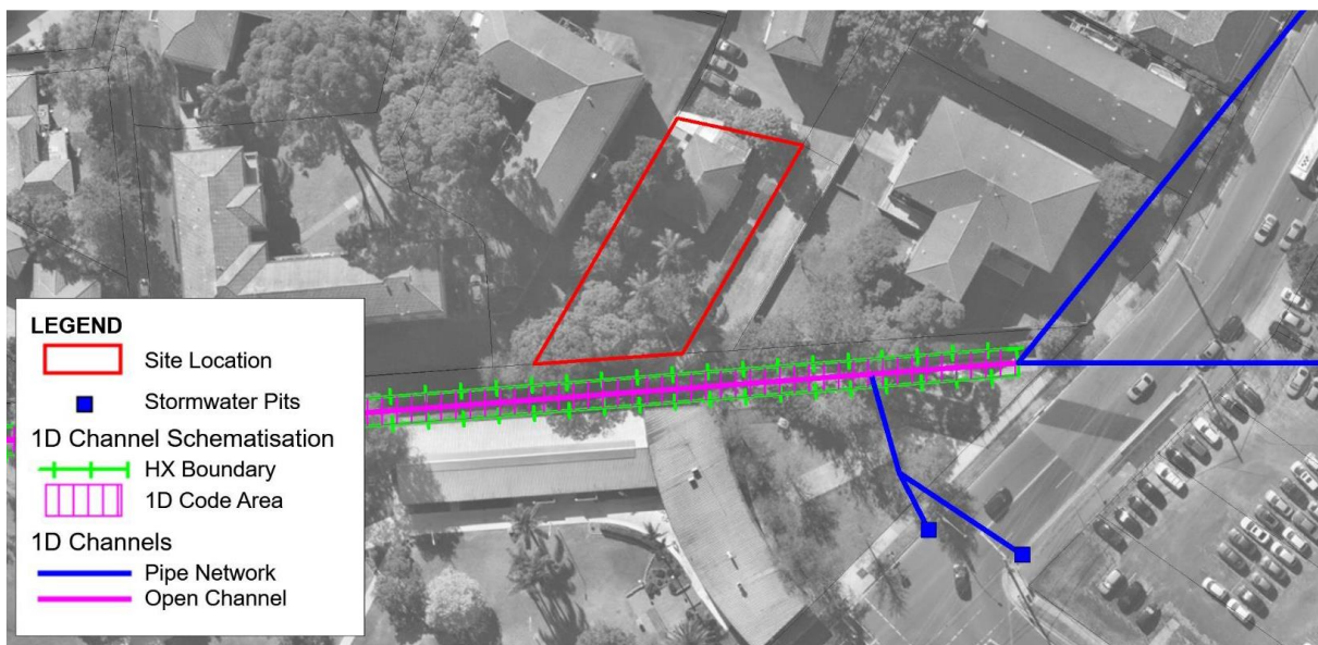
Figure 20 Extract from the Penrith Overland Flood Study TUFLO Schematisation 1D and 2D Models
