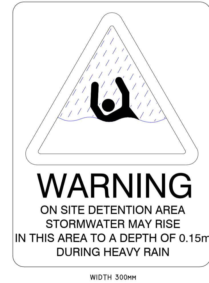
ABOVE GROUND OSD BASIN WARNING SIGN NTS
