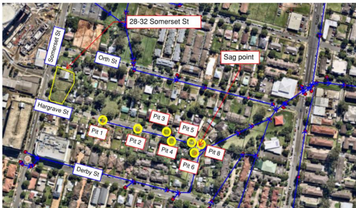
Figure 4 - Existing Drainage System in Hargrave Street
