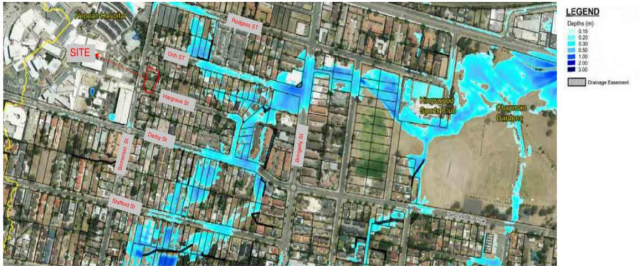
Figure 5 - Peak Design Floodwater Depths for the 5% AEP Flood
