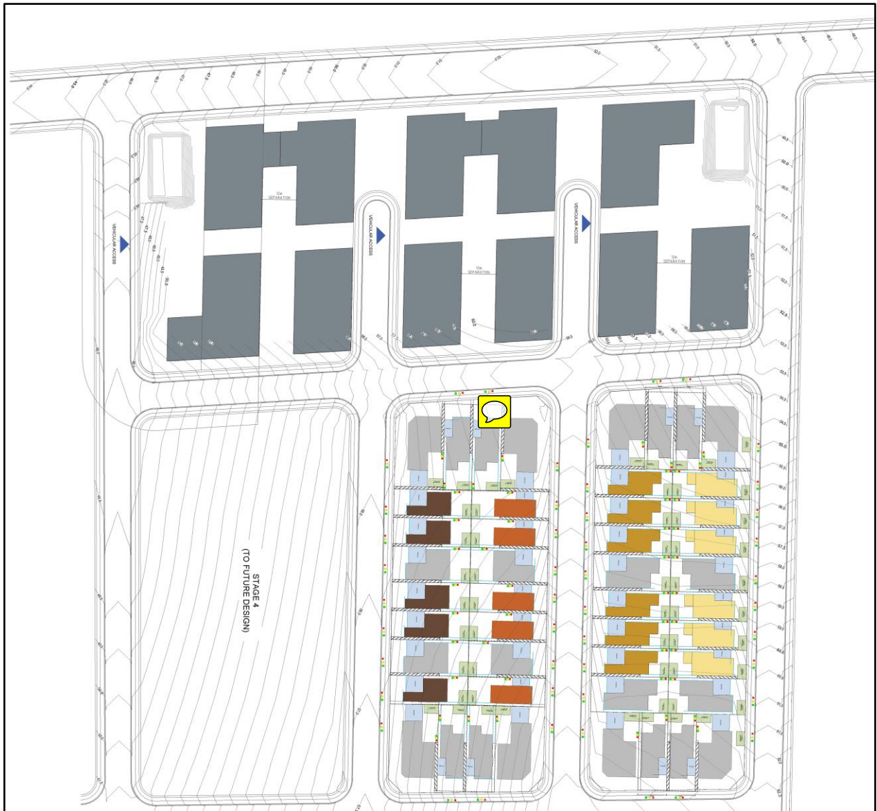
Figure 6: Scaled Diagram of the Waste Storage Areas & Placement for Collection (Western End)
