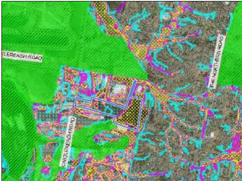
Plate 3 Flood mapping of the Nepean River floodplain, with the study area highlighted in blue; yellow hashing is 20 year flood event, pink hashing is 100 year flood event and blue hashing is probable maximum flood event (Source: Cardno Lawson Treloar Pty Ltd 2006, Figure 6.1 E)
