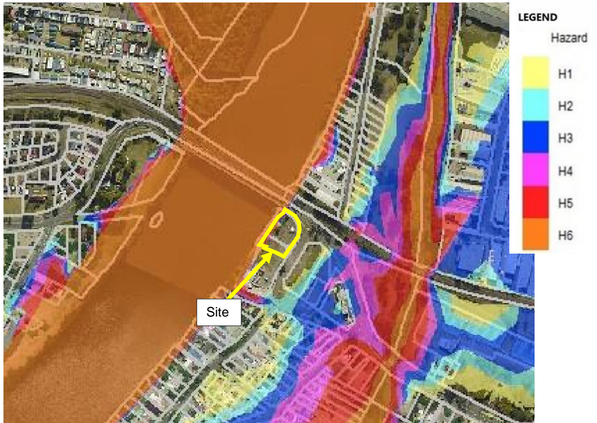
FIGURE 3-5 100 YEAR ARI FLOOD HAZARD CATERGISATION (SOURCE: NRFSFM 2018)
