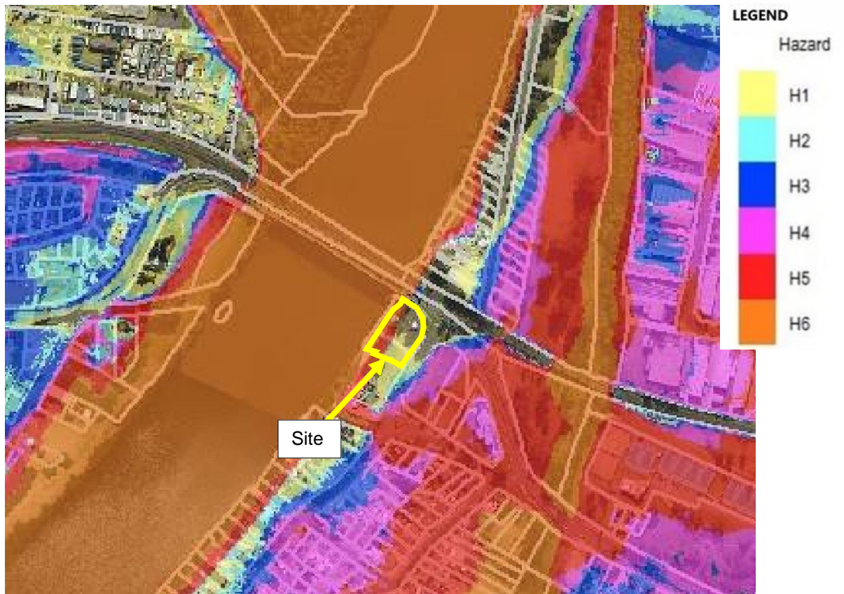
FIGURE 3-6 200 YEAR ARI FLOOD HAZARD CATERGISATION (SOURCE: NRFSFM 2018)
