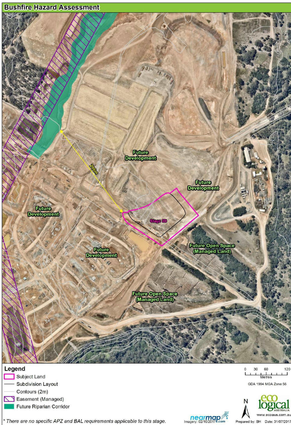
Figure 4: Stage 3d bushfire hazard analysis and separation distances
