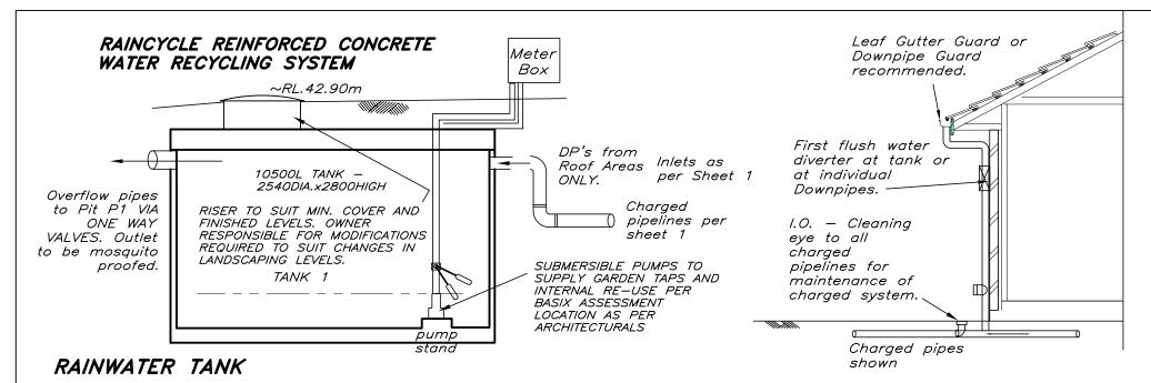
TANK DETAILS SHOWN ARE A SUGGESTED CONFIGURATION ONLY. ANY MODIFICATIONS TO TANK VOLUME OR INLET AND OUTLET LEVELS MUST BE APPROVED BY ENGINEER PRIOR TO COMMENCEMENT OF CONSTRUCTION. TANK SHAPE, & DEVICES SHOWN ARE DIAGRAMMATIC ONLY. MINIMUM OF 450 CLEARANCE (UNLESS L.G.A. REQUIRES LARGER SETBACK) TO SIDE BOUNDARIES MUST BE MAINTAINED. CLIENT IS RESPONSIBLE TO ENSURE COMPLIANCE WITH THIS IN THE INSTALLED STATE.
