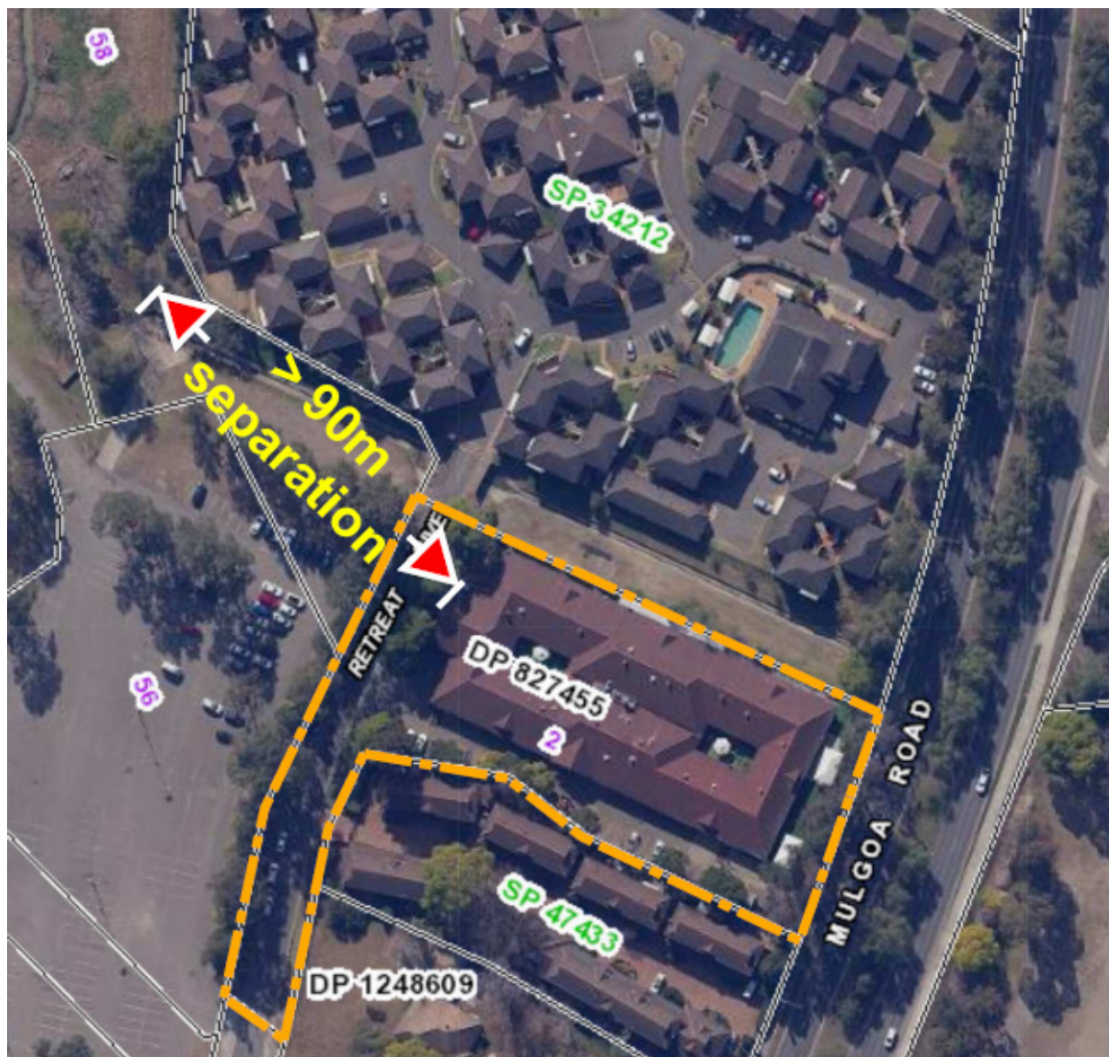
Figure 10 – Plan showing the 90 metre setback to the building, measured from the mapped bushfire prone vegetation in the watercourse located adjacent to the western corner of the Mountain View Retreat Retirement Village.
