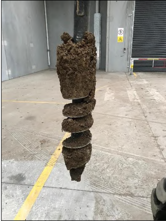
Plate 7 – Fill material encountered.
