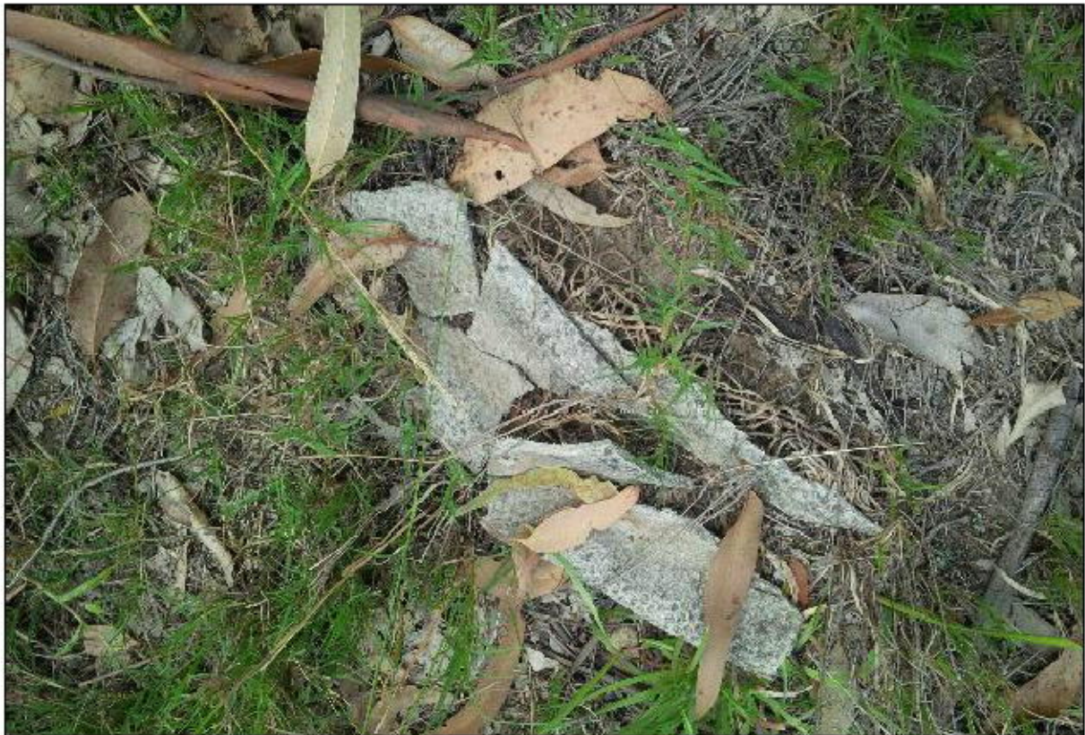
Figure 35. Asbestos containing materials observed on soil surface with area labelled Item 12 on CSM
