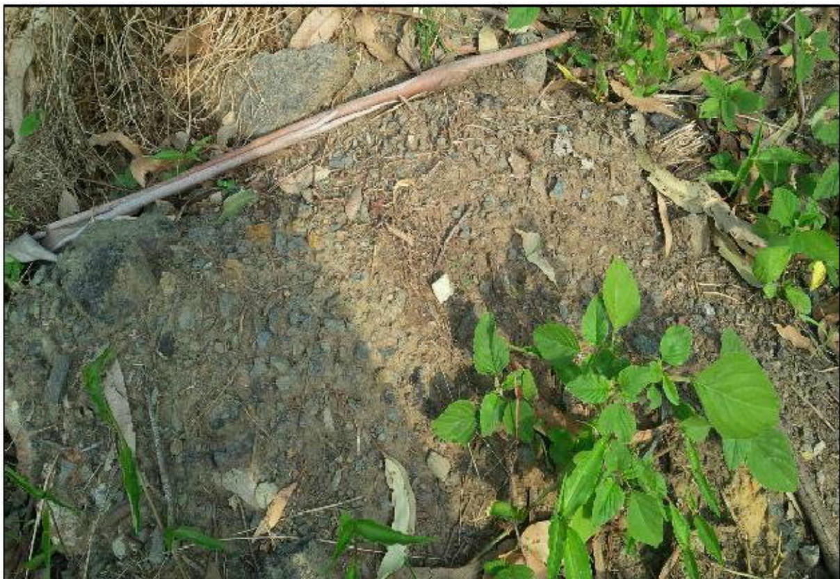
Figure 24. Single piece of asbestos observed on surface of imported fill materials
