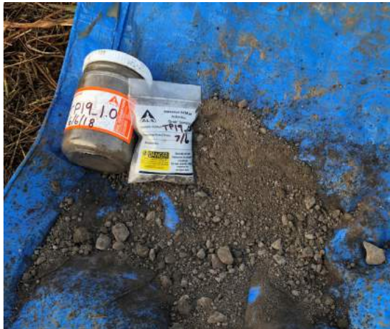
Photo 11: Silty material present at TP19 at 1.0 m
