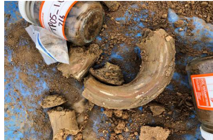
Photo 12: Stiff clay material in TP05
