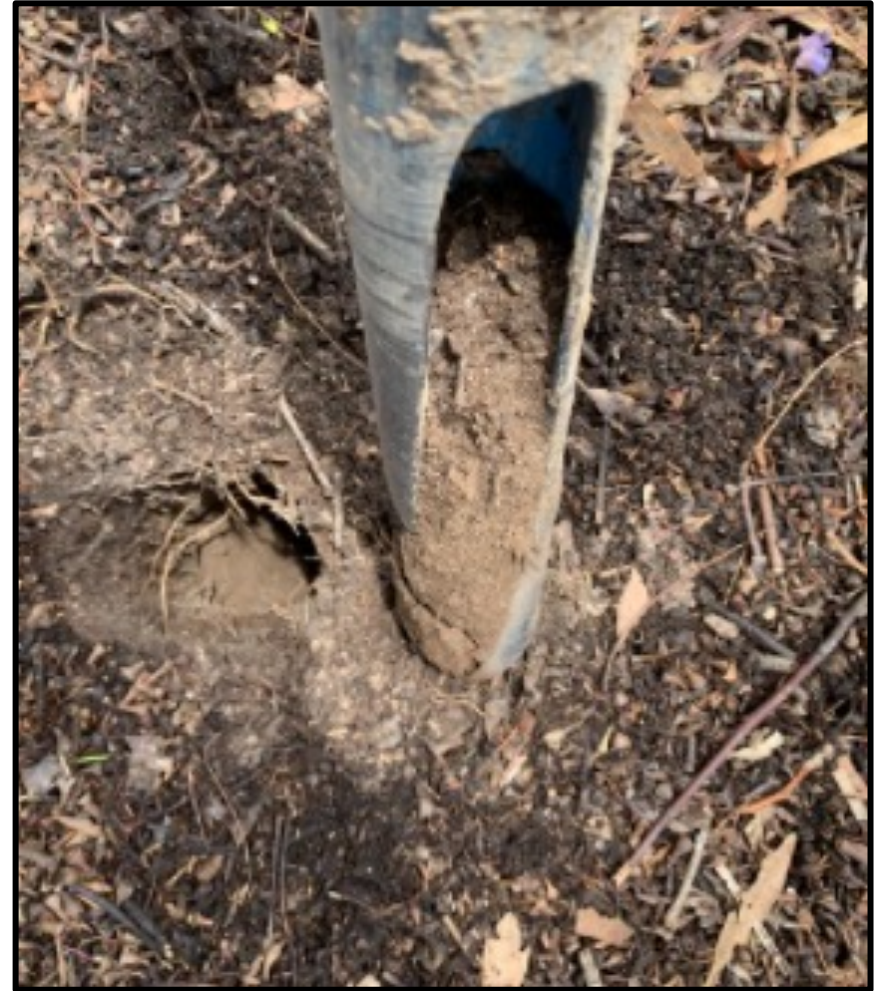
Figure 12. The soil profile of BH2. The soil is dry loam clay.
