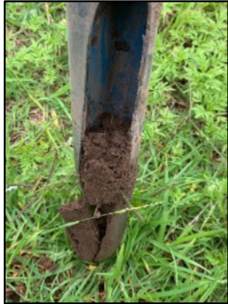
Figure 14. The soil profile of BH4. The soil is moist loam clay.
