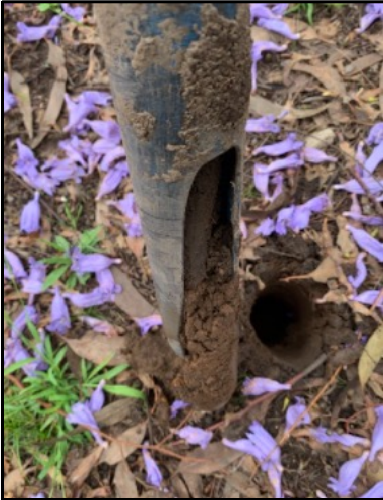
Figure 11. The soil profile of BH1. The soil is moist loam clay.
