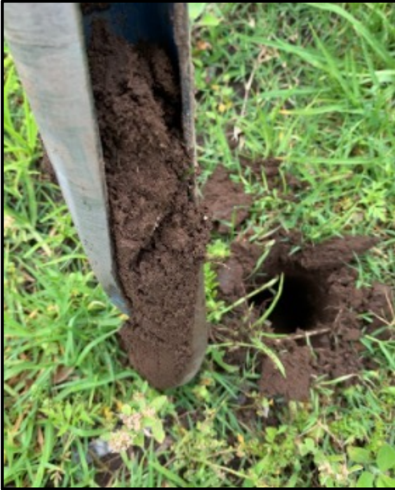
Figure 13. The soil profile of BH3. The soil is moist loam clay.
