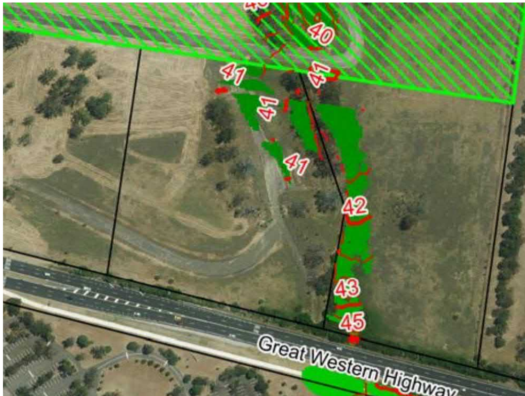
Figure 2-1 1% AEP flood levels - College, Orth and Werrington Creeks Catchment Overland Flow Flood Study (Catchment Simulation Solutions 2017)
