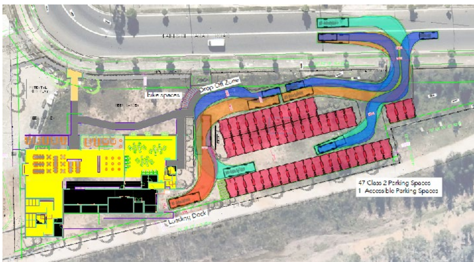
Figure 8 Turning Template Analysis through the site
