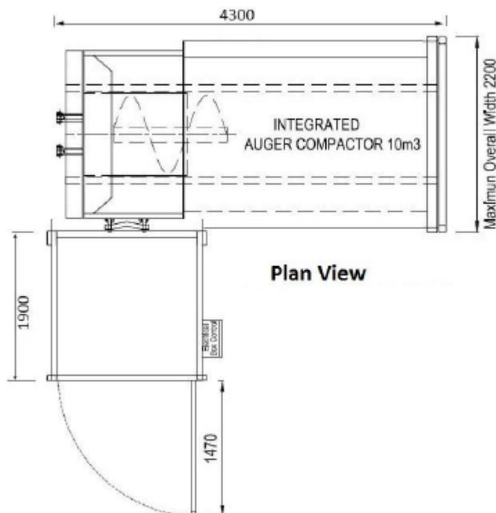
Figure 19: 4.3m Integrated Auger schematic with rear loading bin lifter
