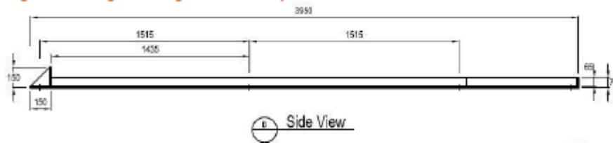
Figure 30: Integrated Auger Guide rails side view
