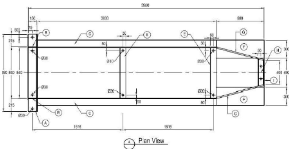
Figure 29: Integrated Auger Guide rails plan view
