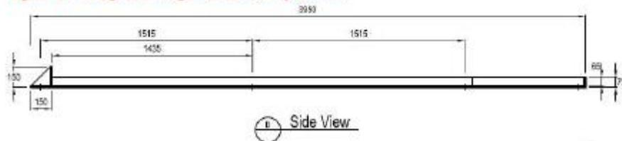
Figure 22: Integrated Auger Guide rails side view
