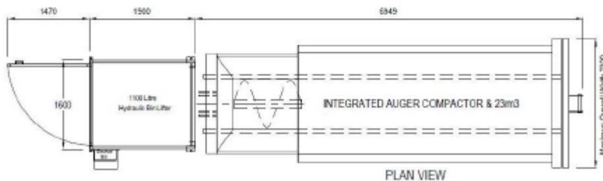
Figure 34: 7.0m Integrated Auger schematic with rear loading bin lifter
