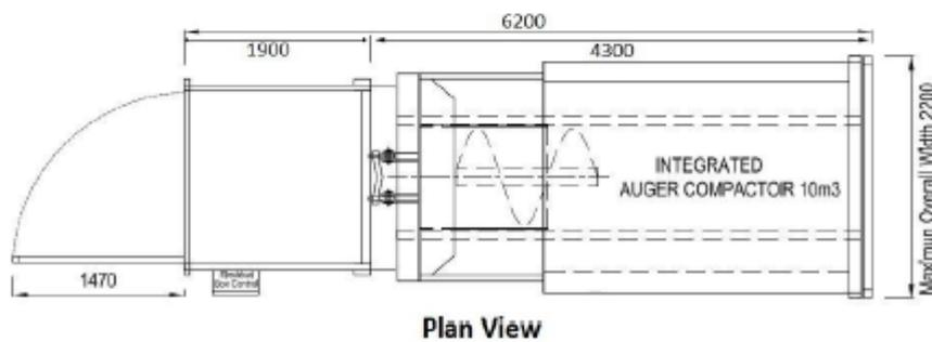
Figure 18: 4.3m Integrated Auger schematic with rear loading bin lifter
