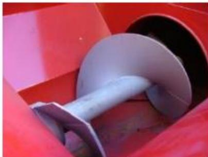
Figure 12: Integrated Auger used to compact objects within the compaction unit
