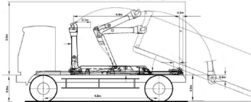
Figure 14: Hook Lift Vehicle ground loading configuration
