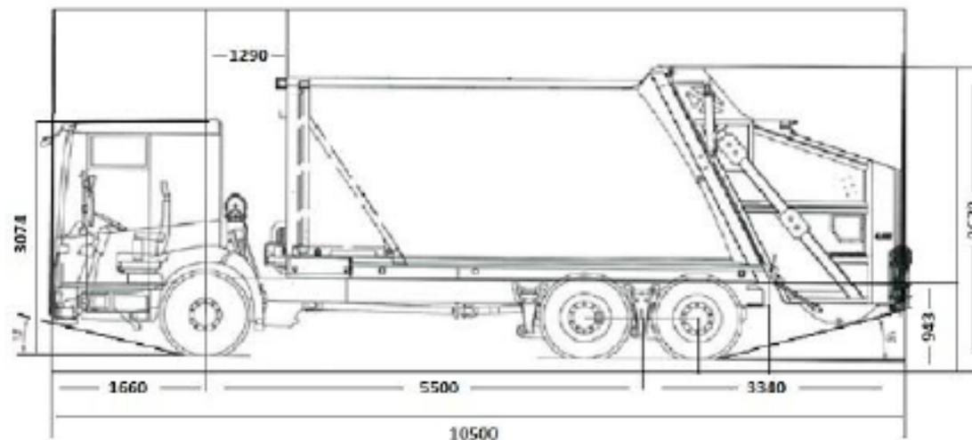
**Figure 5: 10.5m Heavy Rigid Waste Collection Vehicle specifications**
