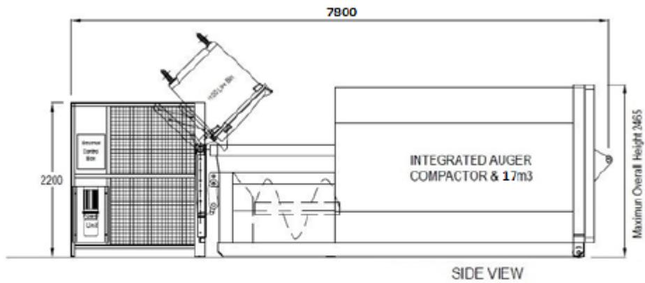
Figure 28: 6.0m Integrated Auger schematic side view
