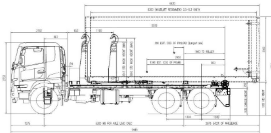
Figure 24: 8.3m Hook Lift Waste Collection Vehicle specifications
