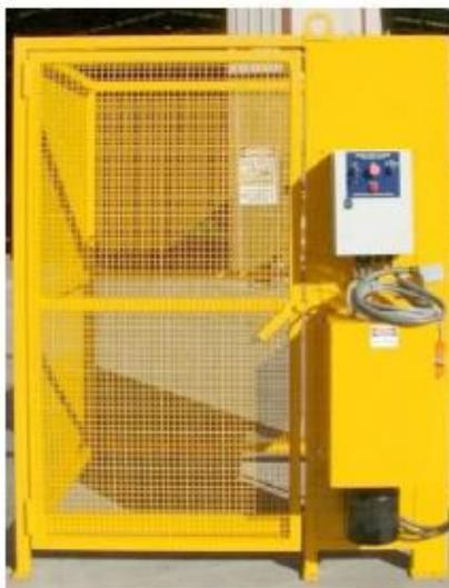
Figure 13: 1100L bin lifter used to empty bin into the Auger Compactor
