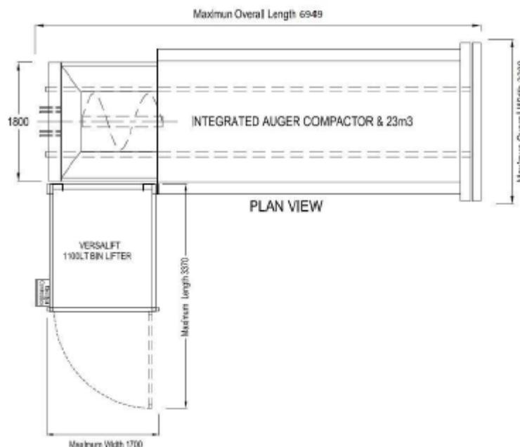
Figure 35: 7.0m Integrated Auger schematic with side loading bin lifter
