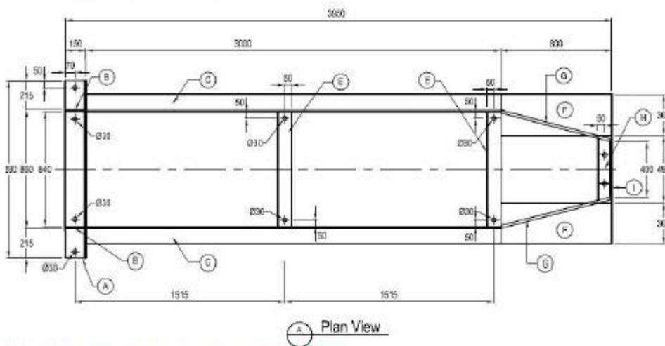
Figure 21: Integrated Auger Guide rails plan view
