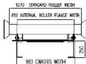
Figure 17: 9.5m Hook Lift Waste Collection Vehicle tray specifications
