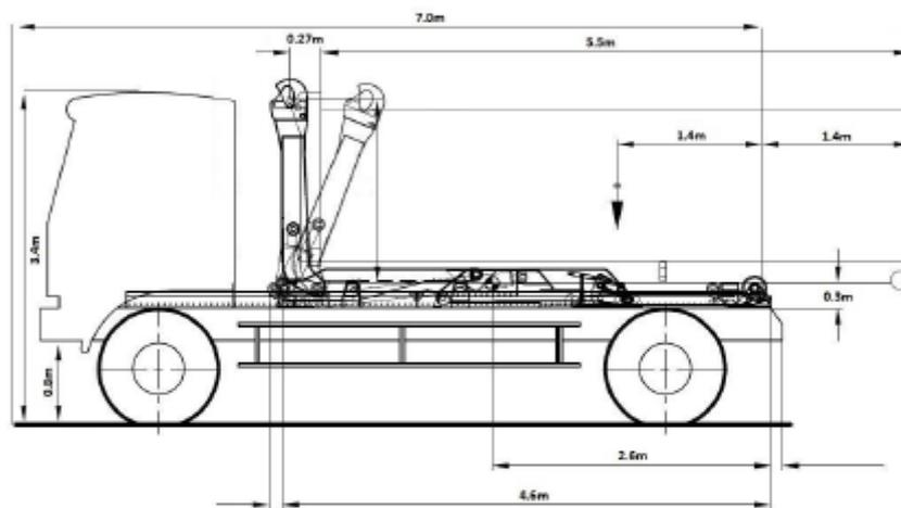
Figure 16: 7m Heavy Rigid Waste Collection Vehicle specifications
