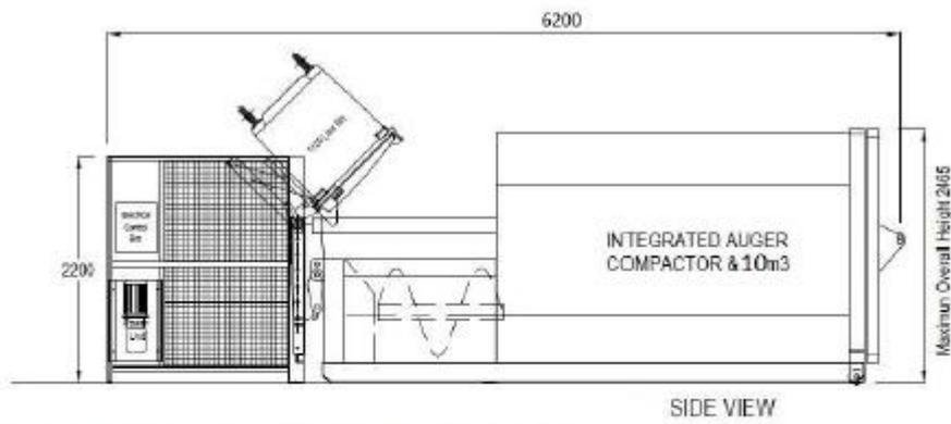
Figure 20: 6.0m Integrated Auger schematic side view
