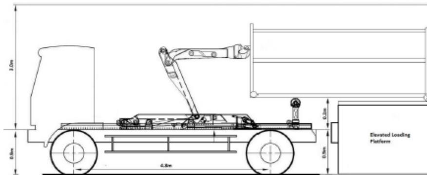
Figure 15: Hook Lift Vehicle ground loading configuration
