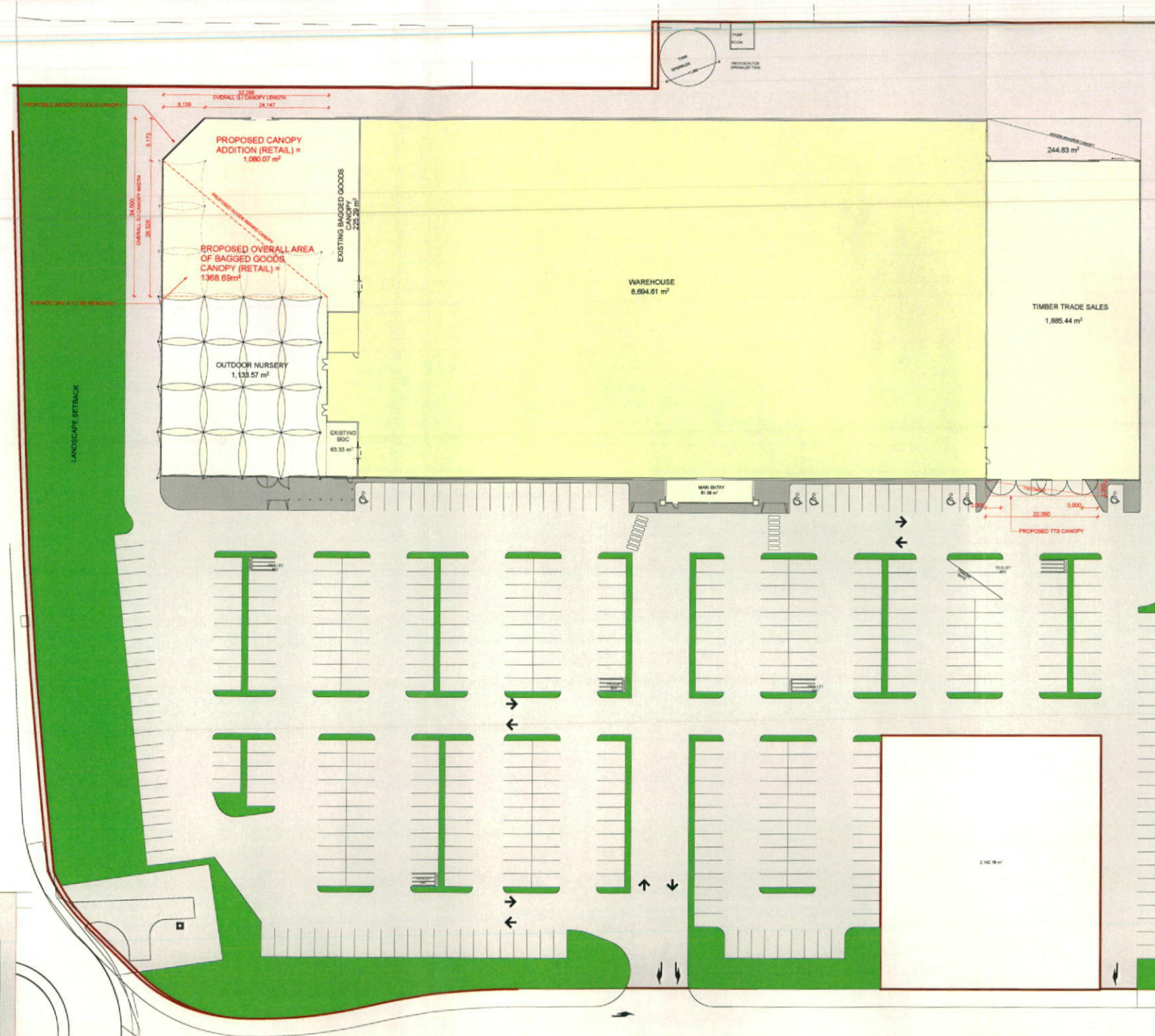
PROPOSED BAGGED GOODS CANOPY SCALE: 1:500 @ A1
