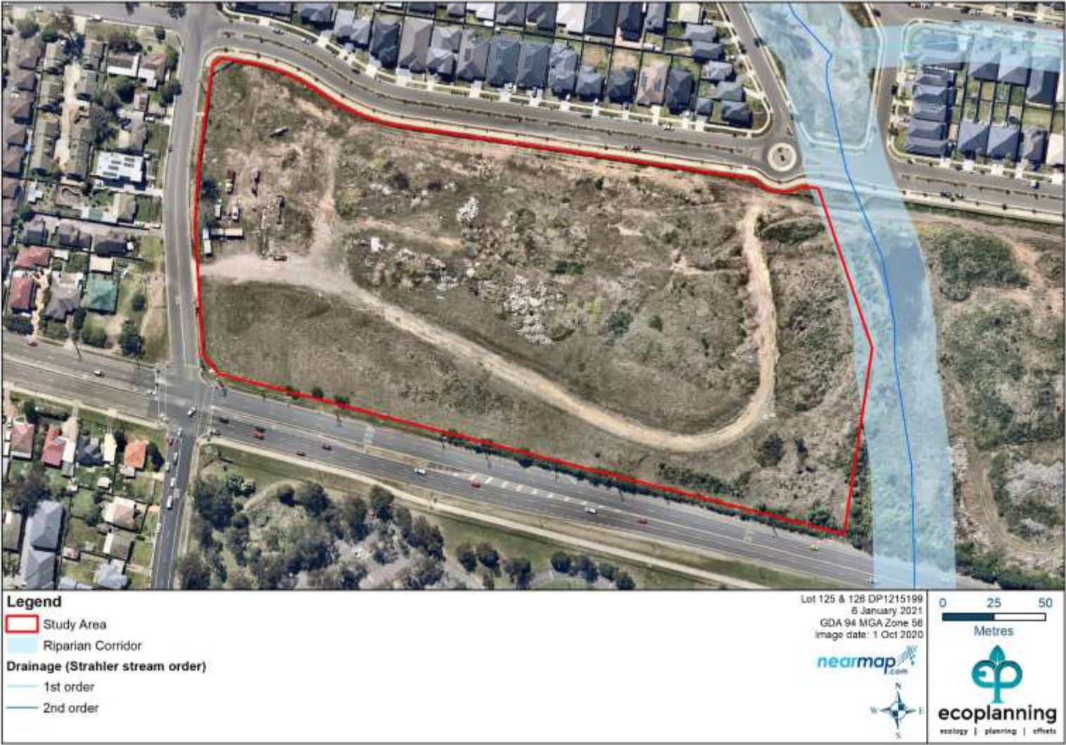
Figure 3.3: 20 metre buffer (40 metre wide corridor) required for a VRZ around the second order stream on the site
