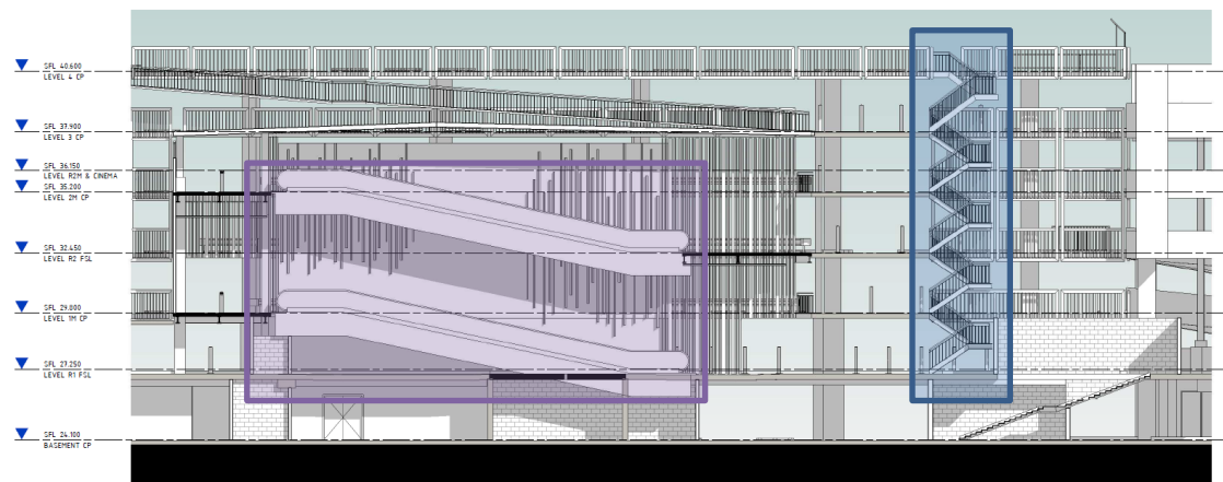
Figure 7-3: Section drawing showing the proposed travelators and emergency egress stairway
