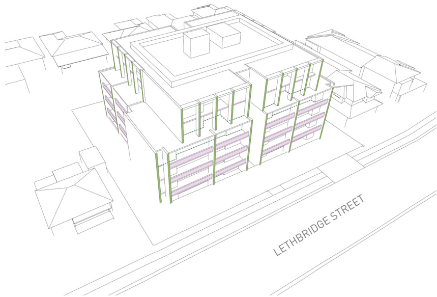
Built Form Diagram 3. A Vertical and horizontal language is developed to express dividing walls and balconies. Vertical elements are repeated on upper levels and horizontal elements reduced to give a thinner less bulky appearance.
