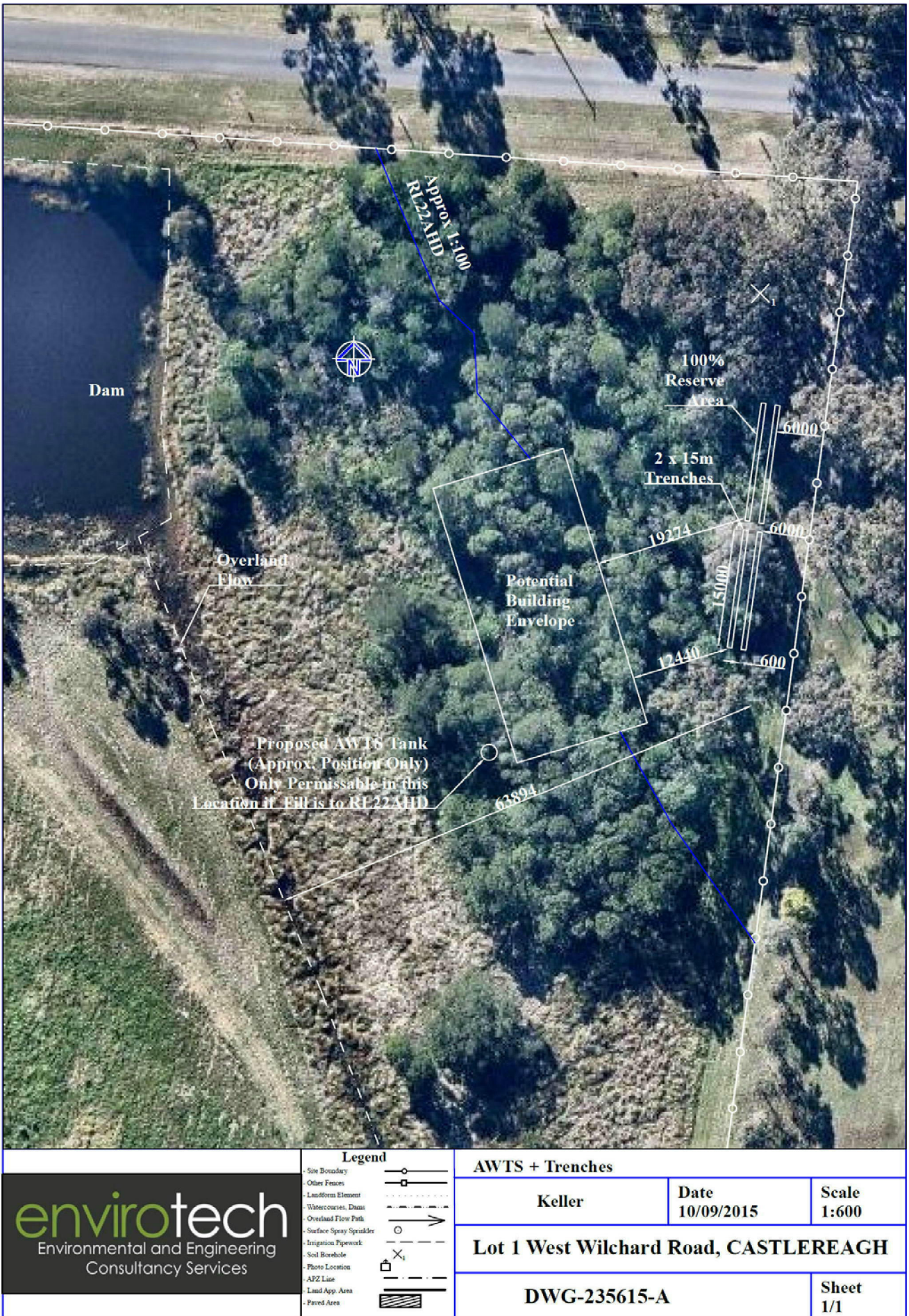
Figure 3: On site wastewater management system design.
