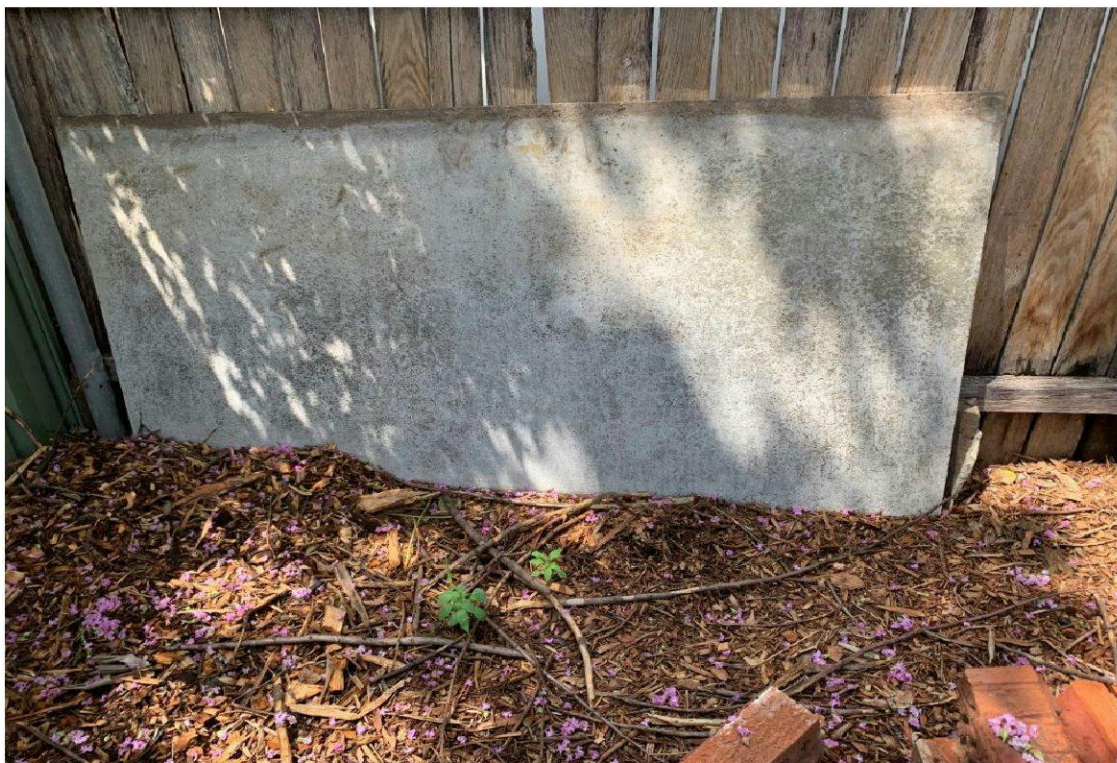
Photo 9 - 40 Orth Street, Fibre cement sheet along back fence potentially containing asbestos
