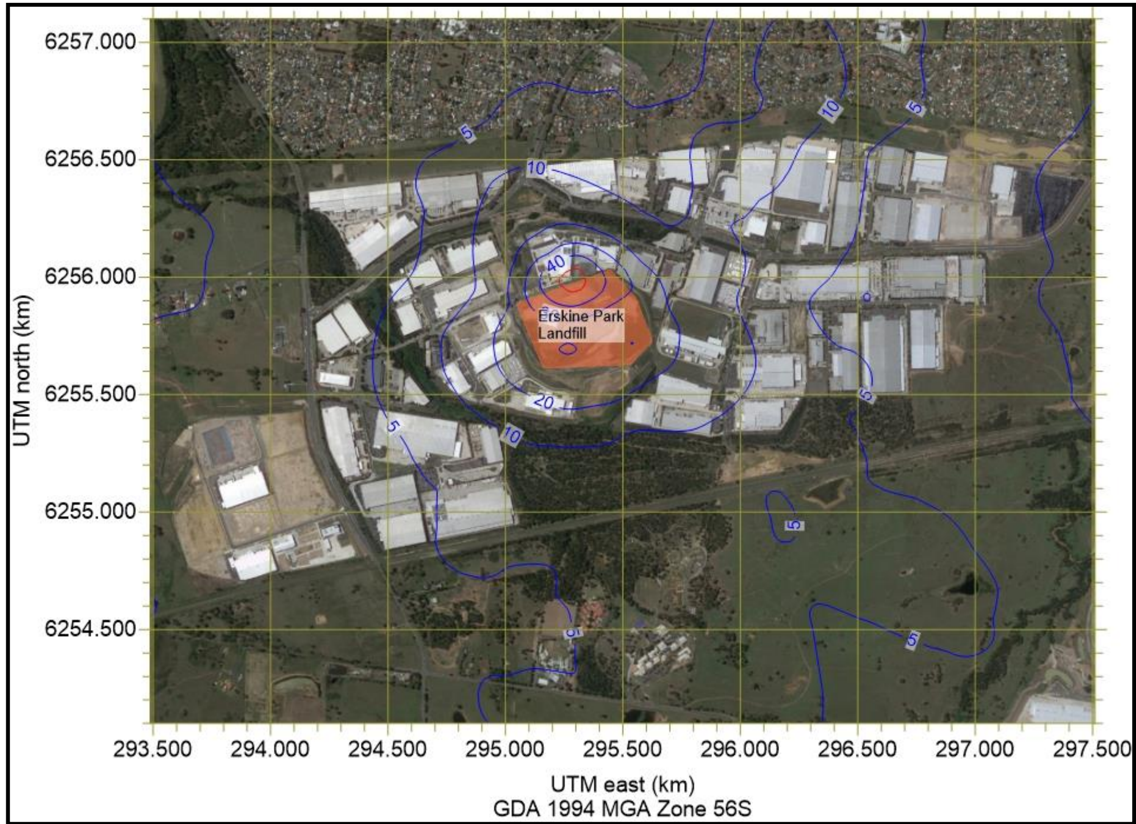
Figure 5.4 – Contour plot showing predicted maximum 24-hour average ground-level PM 10 concentrations (µg/m 3 ) due to Erskine Park Landfill operations
