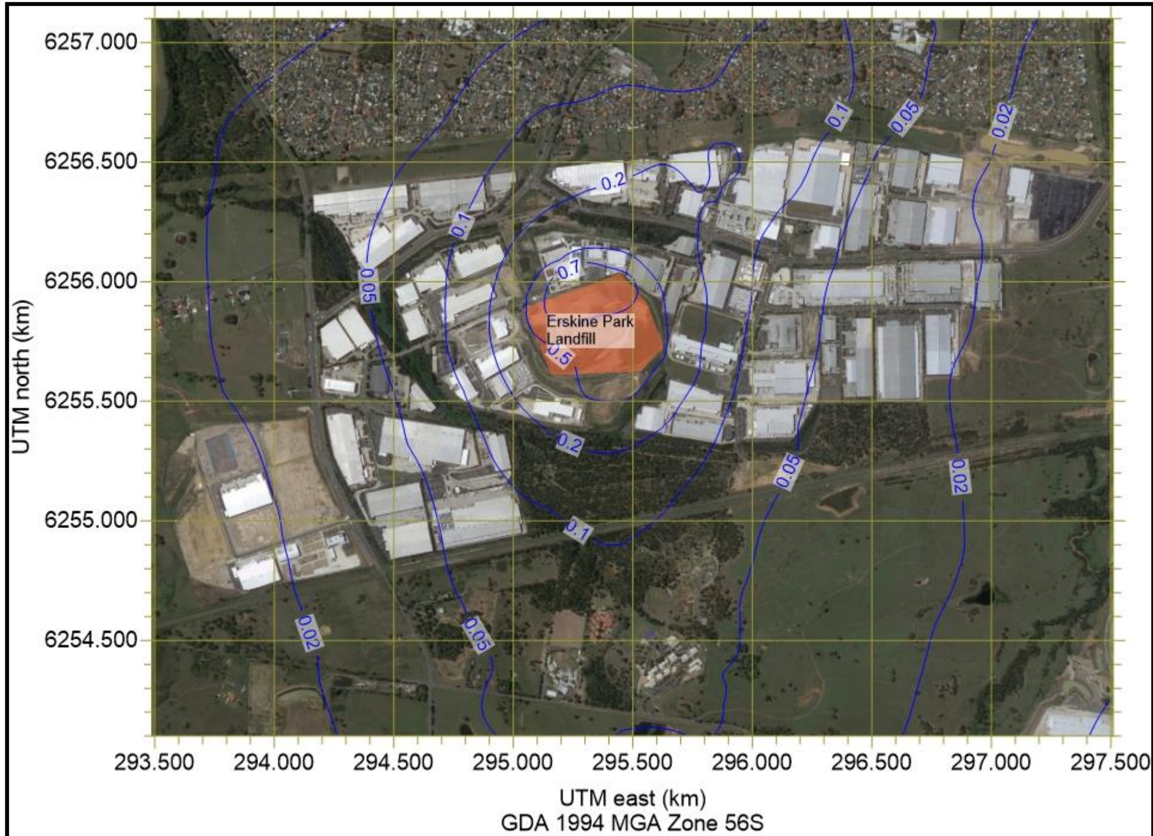
Figure 5.7 – Contour plot showing predicted annual average ground-level PM 2.5 concentrations (µg/m 3 ) due to Erskine Park Landfill operations
