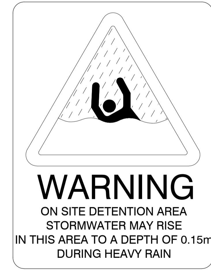
ABOVE GROUND OSD BASIN WARNING SIGN
