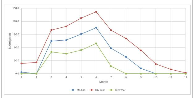
Peak irrigation in a hot dry year is estimated to be 142 kL/irrigation. Assuming the irrigation flow rate of 420 L/min this can be achieved in 5.6 hours, achievable within the 7-hour window of operation.
