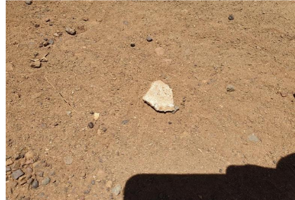
Photo 2 - Potential ACM observed on the surface of fill in an access way
