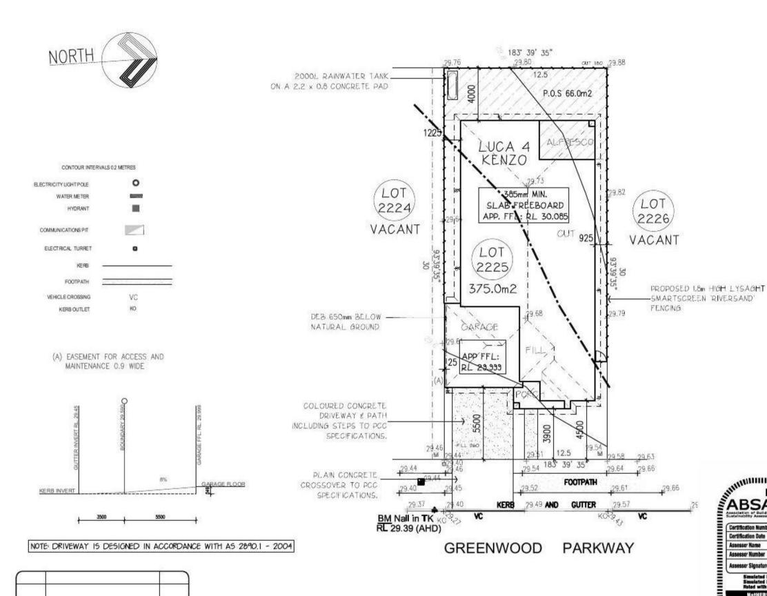
**CUT & FILL BUILDING AREA TO** RL 29.7 APPROX. TO CREATE LEVEL **BUILDING PLATFORM FOR** WAFFLE POD SLAB
