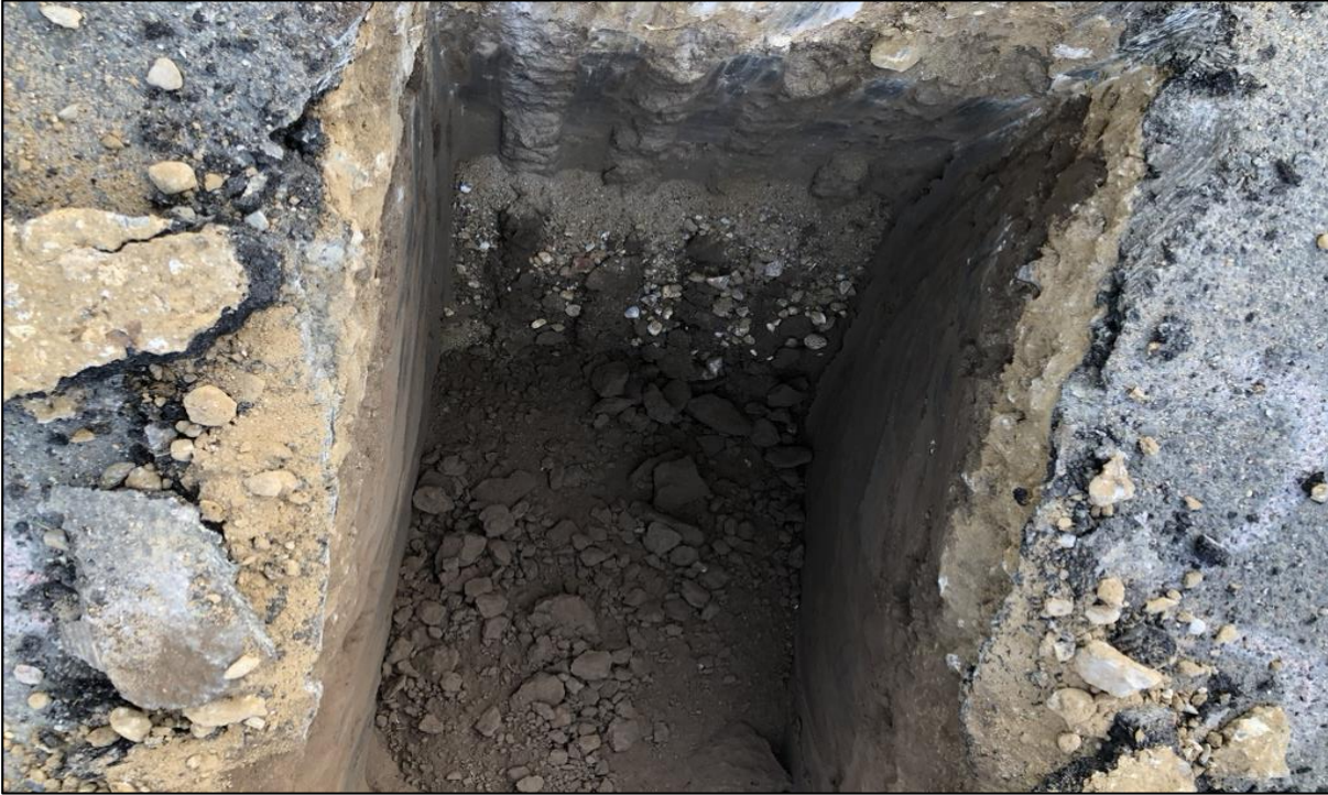
Photograph 2. Soil materials as observed under asphalt in eastern carpark – Test Pit CC78.
