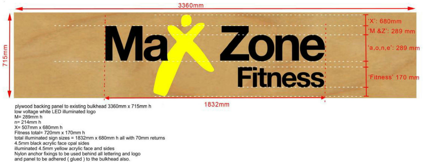
Figure 11b – shows panel, lettering & sign dimensions
