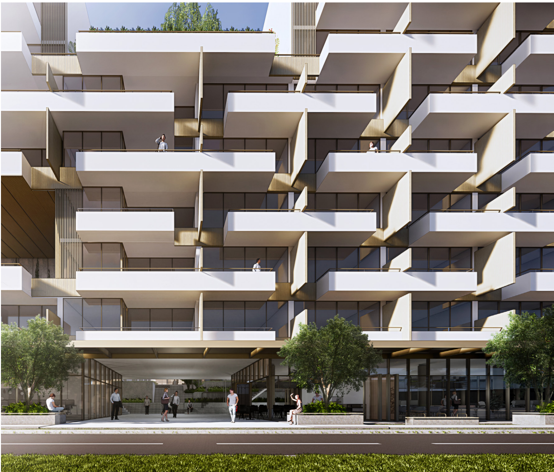
Facade depth to achieve solar protection
