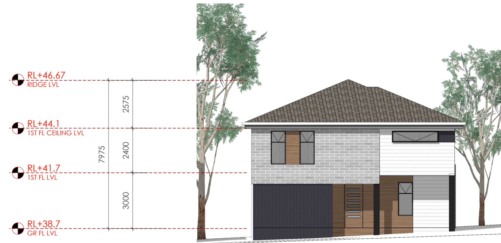
FRONT (EAST) ELEVATION
