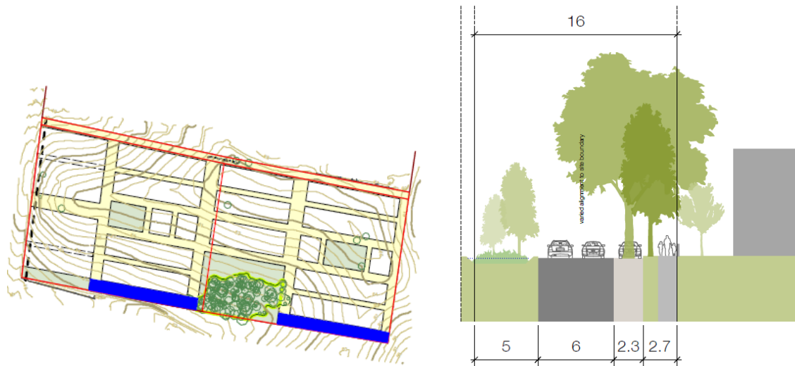
Figure 12 16m Wide Road – Edge Corridor (Hills Thalys)
