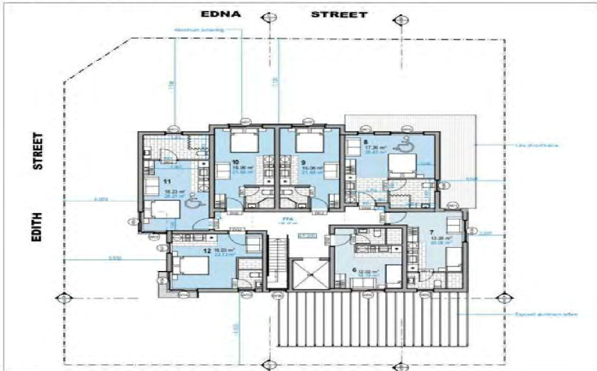
Figure 7: First Floor Plan Source: Designcorp Architects
