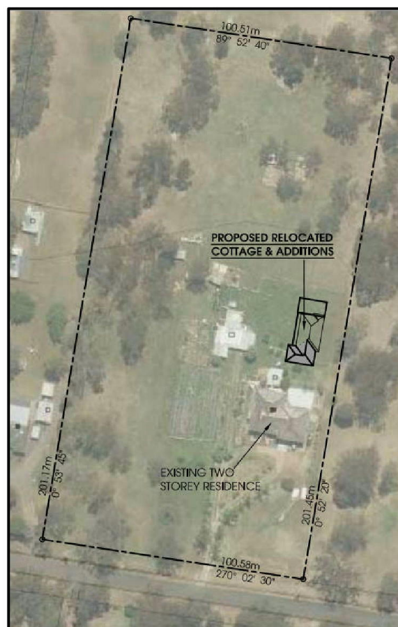
Figure 13 Site plan for relocated dwelling and additions
