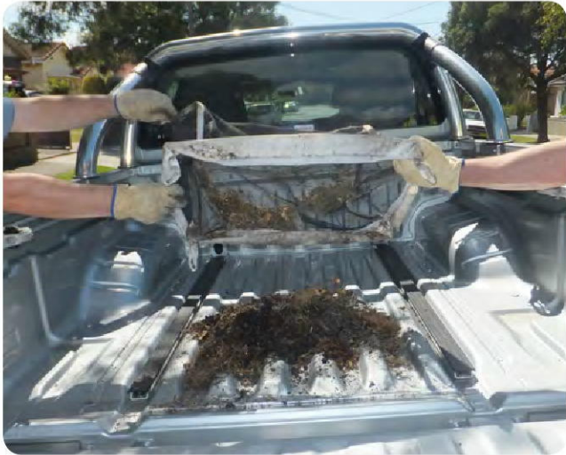
Photo 25 Slightly clogged filter bag, indicated by the brown stain on in the centre of the bag
