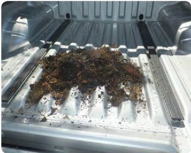
Photo 18 Completely empty the contents of the filter bag
