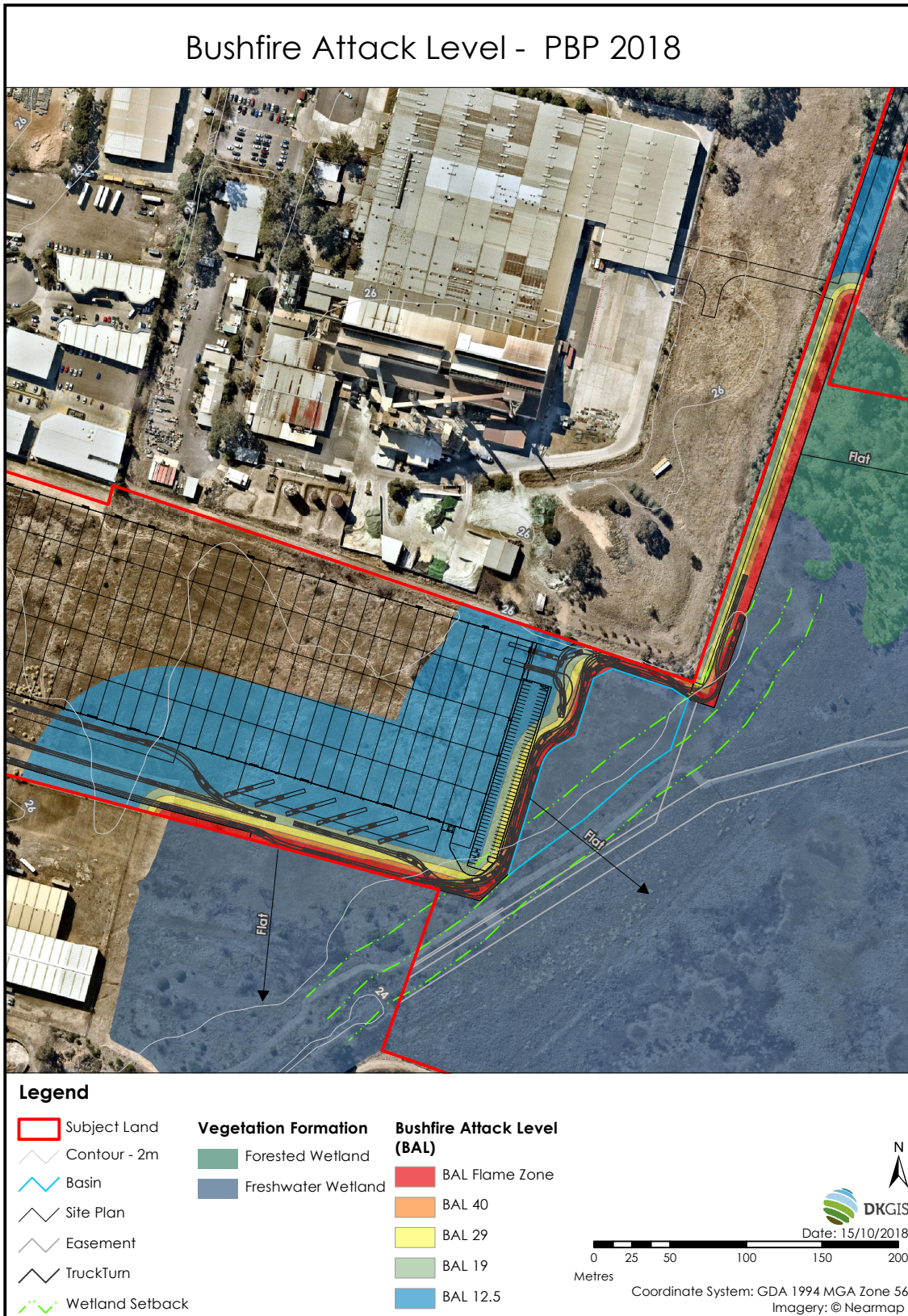
Figure 8 Bushfire Attack Levels on the proposed warehouse
