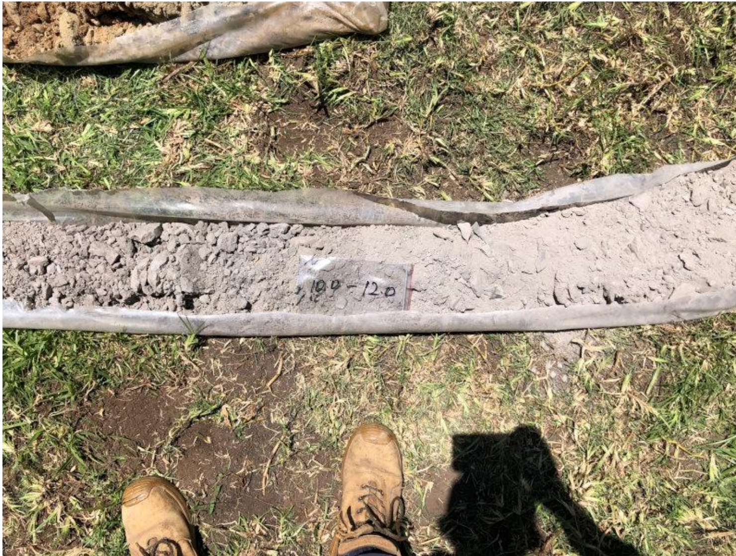
Rock Cutting from BH2 Depth 10.0-12.0m
