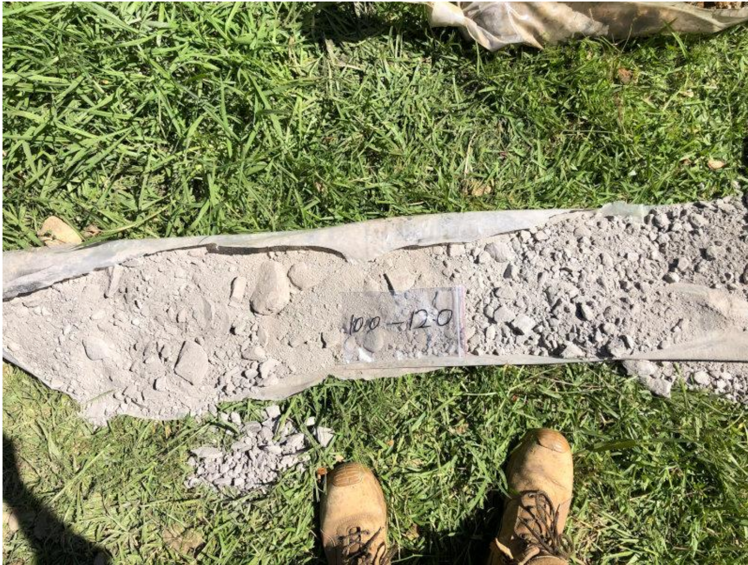
Rock Cutting from BH1 Depth 10.0-12.0m
