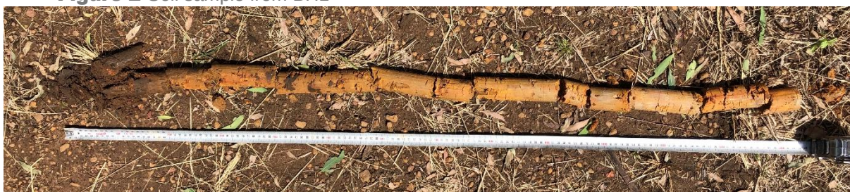
Figure 2 Soil sample from BH1
