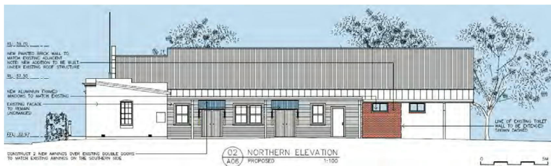
24. Proposed North Elevation- new works coloured (Source: JLD dwg. A06 [NTS]).
